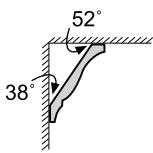
When the ceiling strips/mouldings are to be sawn lying flat on the saw table, the standard mitre angles of 31,6° (horizontal) and 33,9° (vertical) must be set. The following table contains instructions for sawing ceiling strips/mouldings.
